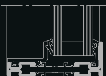
Glasleiste Winkel Angled glazing bead
