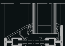
Glasleiste Schräg Inclined glazing bead
